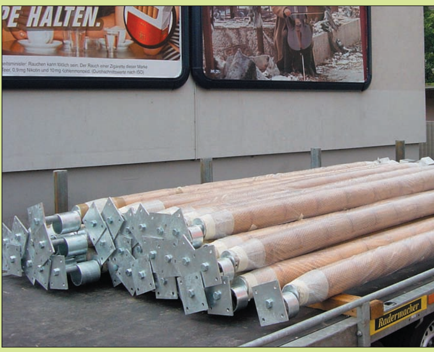
33 Bamboo Poles as loadbearing structure
